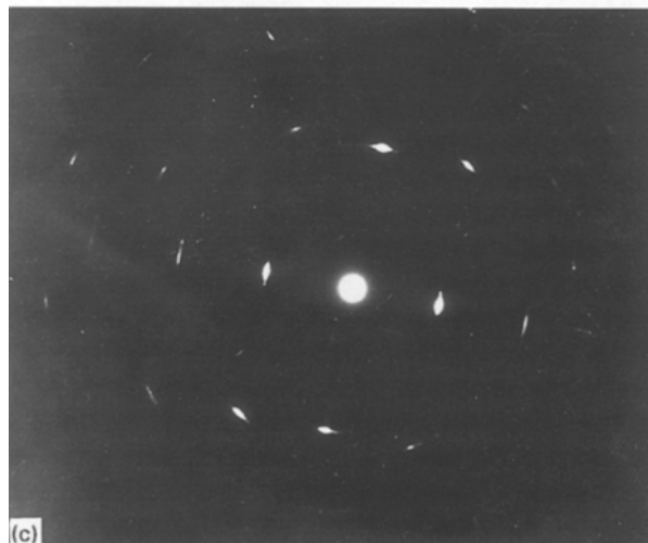
Figure 6 Selected area electron diffraction patterns near the position S indicated in Figure 4, representing (A) (1 1 1) plane, (B) (2 0 0) plane, and (C) (4 2 2) plane of an fcc crystal having a lattice parameter of 0.360 nm. (Accelerating voltage = 200 keV, camera length = 100 cm).
